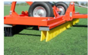
**Granulate loosening brush for artificial turf**
