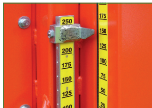
Tool-free adjustment of the tine angle and the working depth with the QuickSet feature.
