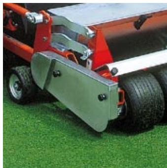
Belt drive for the stirring shaft.
