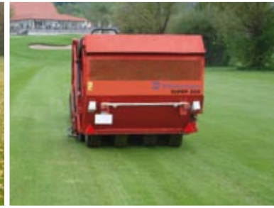
Verticutting Verticutting with simultaneous collecting of material. Verticutting spacing ¾", 1½" or 2¼"
