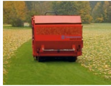
Sweeping / collecting leaves Collecting grass clippings or leaves without damage to turf by means of brush-type head or multi-purpose sweeper head.
